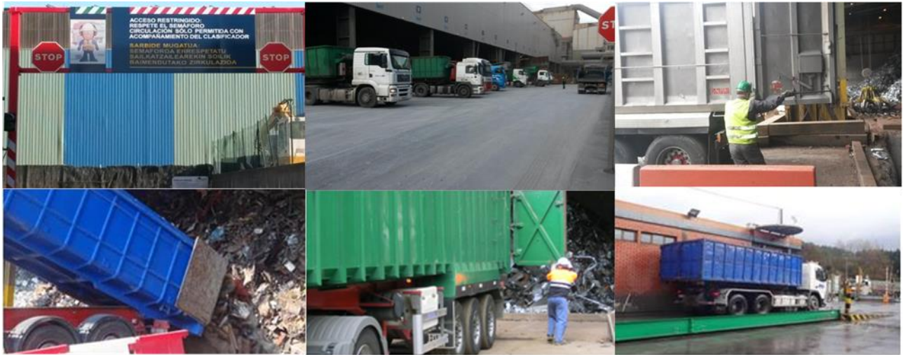
Illustration .Current process implemented at Sidenor when receiving, classifying and processing scrap metal
